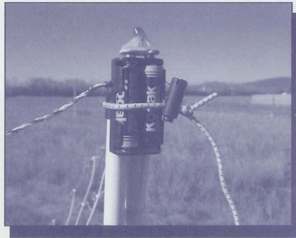
Figure 4—LEDs (light-emitting diodes) attached to two sides of a portable electric mesh fence can warn campers or animals before they touch or run into the fence.
