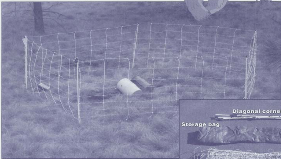
Figures 1—This portable mesh electric fence is a potential alternative for storing food, garbage, and other attractants in bear country. The fence kit weighs just 9 pounds with the diagonal braces and 7 pounds without the braces. The posts are 42 inches long.
